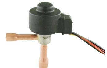
LPF series Electric Expansion Valves are designed for use in refrigeration systems. The valve port is designed with PTFE (Teflon™), creating a tight seat equivalent to a solenoid valve thus preventing liquid refrigerant from migrating to the evaporator and compressor.
