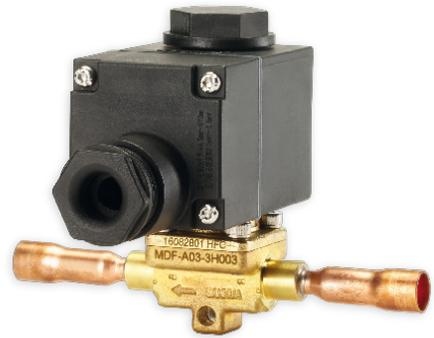
MDF series solenoid valves are direct operated or pilot operated solenoid valves, mainly used in refrigerant control of various devices such as refrigerating and freezing systems, air conditioners and heat pumps. All the Solenoid Valves listed in this datasheet can be installed in system using flammable refrigerants HFO (categories A2\* and A2L\*), and Hydrocarbons HC (category A3\*).
