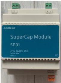
Ultracap Ultracapacitor to close the valve if main supply cuts off
